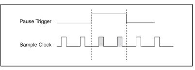
Figure 5-5. ao/PauseTrigger with Other Signal Source
